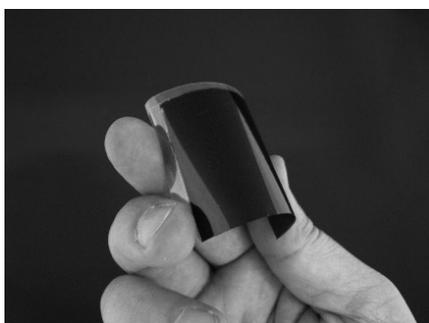
Fig. 1 Flexible and adhesive CNT sheet.
