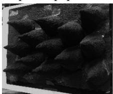
Fig. 3 Photo of a pyramid type MW absorber made by NT composite paper.
