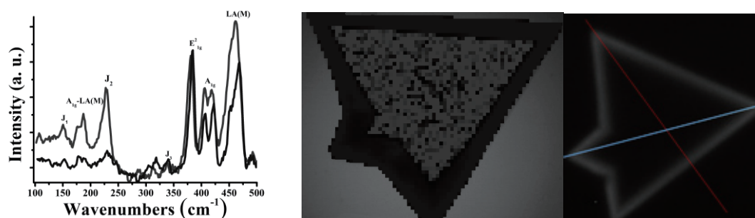
Fig.1. (a) Raman at the basal plane (gray) and at the edges (black), (b) Raman mapping showing the superposition of J 2 peak (gray) and E 2g intensities and (c) PL intensity map of in plane MoS 2 heterostructure.
