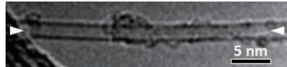
Fig. 1 TEM picture of a long LCC inside SWCNT.
