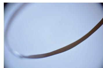
Fig.2 A ring of a curved DND whisker.
