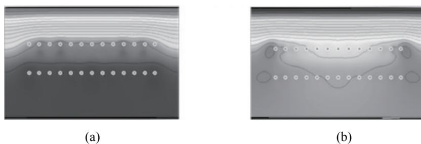
Fig. 1 Contour plots of the electrostatic potential of the bilayer a GNRs with AB stacking arrangement under the electric field injecting excess (a) 0.1h and (b) 0.1e . The gray circles denote C atoms.
