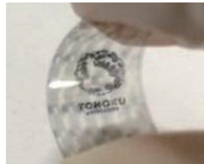
Fig. 1. Optical image of a transparent and flexible solar cell fabricated with TMD.
