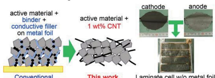
Fig. 2. CNT-sponge-based lithium ion battery [8].
