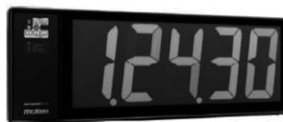
Fig.2 Commercialized product of E-paper using Toray DWCNT TCF
