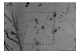
Fig 4: Optical image of single layer graphene coated Cu
