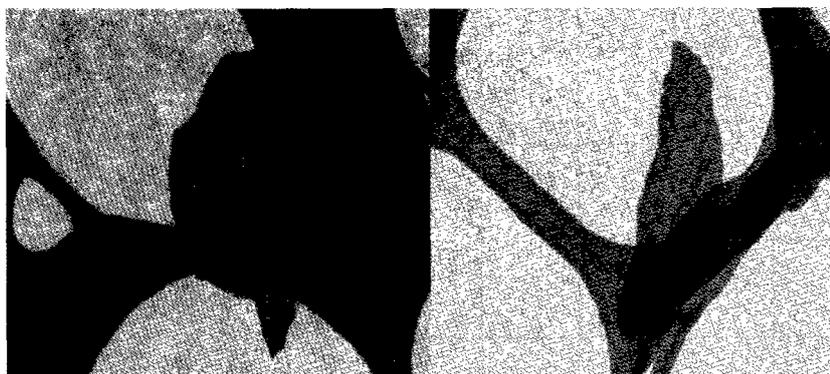
**Fig. 2** STEM images of polyglycerol-functionalized graphene
