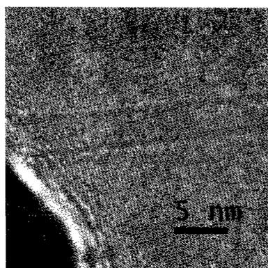
Fig. 1 TEM image of a suspended DWCNT.
