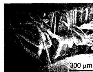
Fig. 1 Aligned carbon nanotubes with graphite roof.
