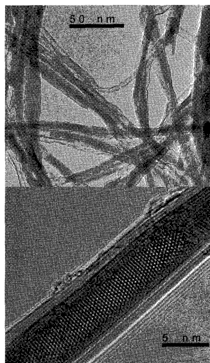
Figure 1. HR-TEM images of AgI@MWCNTs
