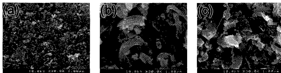
Fig.1. SEM micrographs of electrodes. (a) AcB, (b) CNC, (c) crushed CNC
