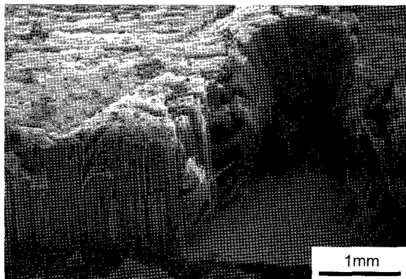
Fig.1. SEM image of 2 mm long vertically aligned CNTs on quartz substrate.
